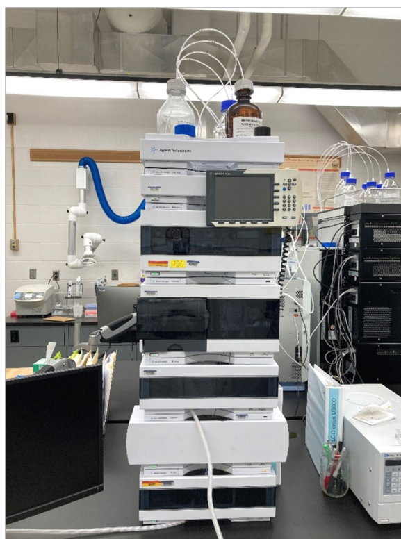
'Agilent 1260' = Agilent Technologies 1260 Infinity HPLC System with Diode Array Detector
