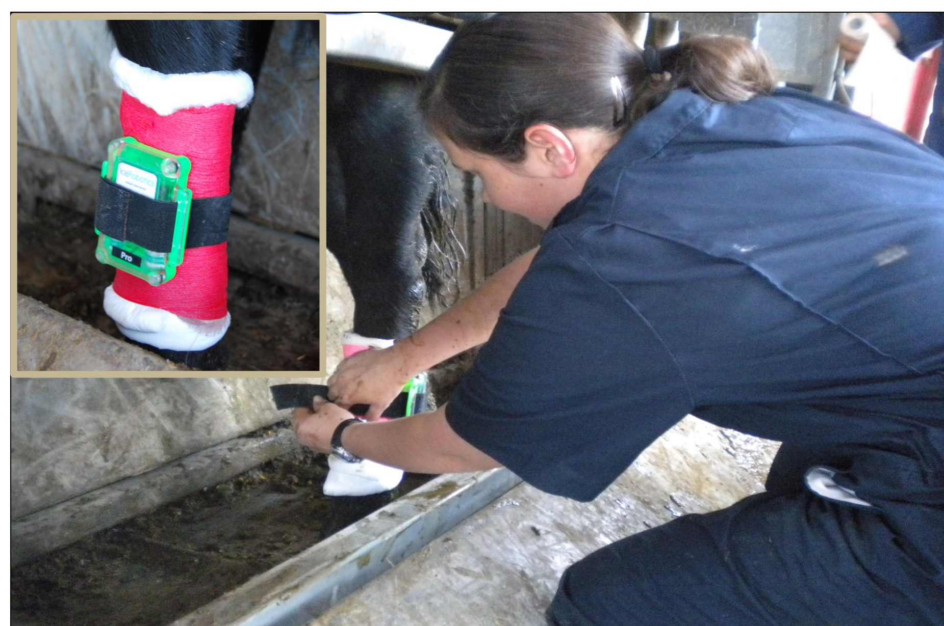
Figure 2. ICETag 3D Accelerometer secured to the left hind leg of each heifer for a period of 7 days to record locomotion and length of time lying down.
