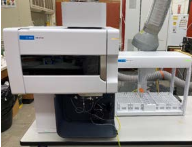
'ICP-OES 5800' = Agilent Technologies ICP-OES System
