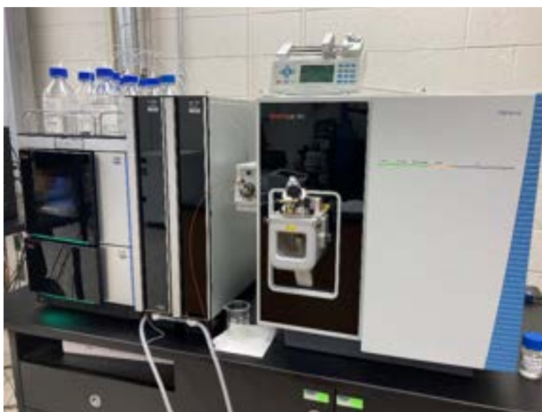
'Altis 3' = Thermo Fisher Scientific TSQ Altis Triple Quadrupole Mass Spectrometer with Vanquish UHPLC System
