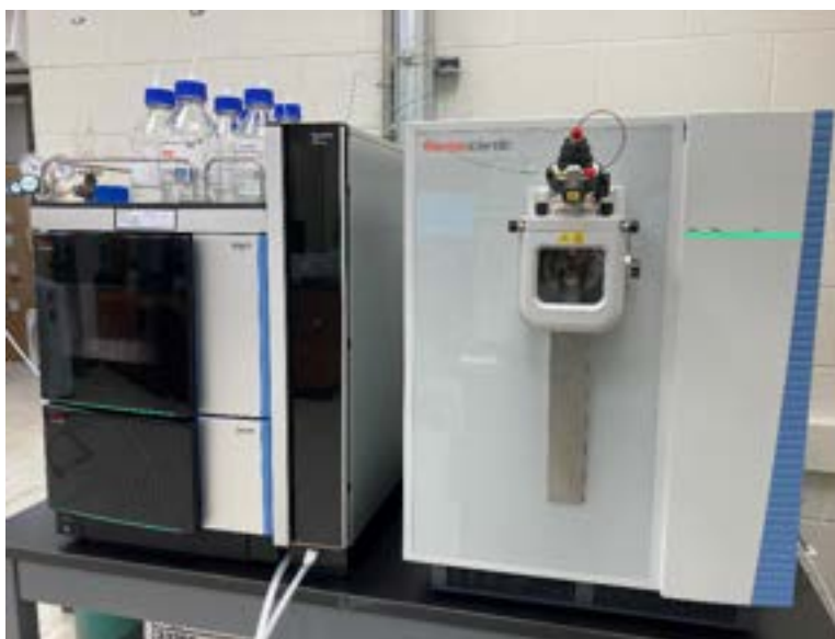
'Exploris 120' = Thermo Fisher Scientific Exploris 120 Mass Spectrometer with Vanquish UHPLC System
