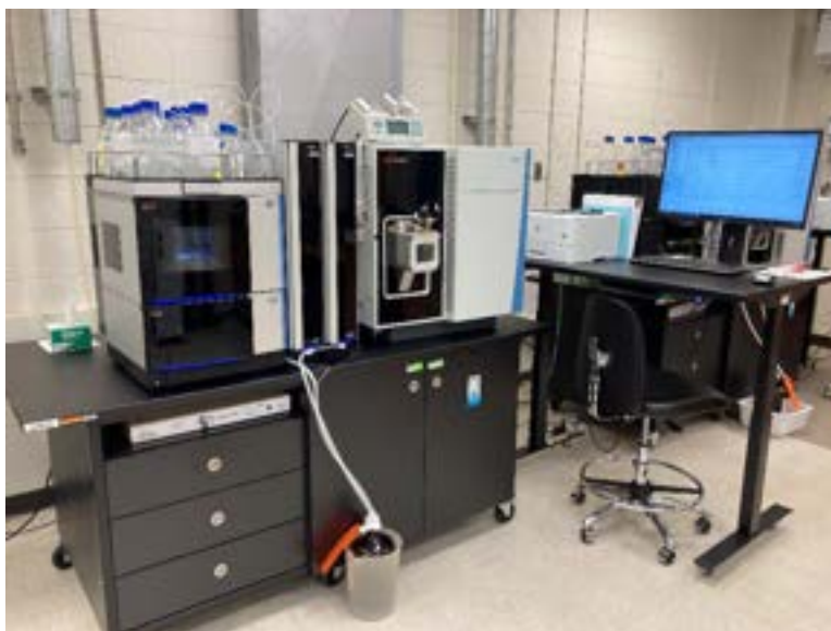
'Altis 2' = Thermo Fisher Scientific TSQ Altis Triple Quadrupole Mass Spectrometer with Vanquish UHPLC System
