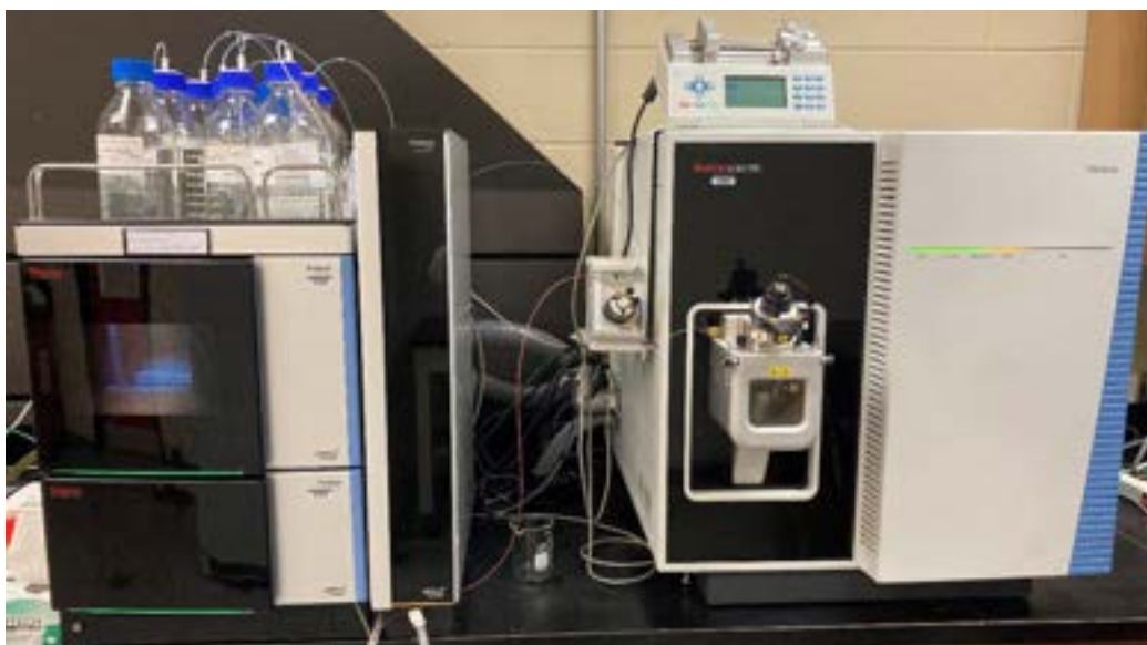
'Altis 1' = Thermo Fisher Scientific TSQ Altis Triple Quadrupole Mass Spectrometer with Vanquish UHPLC System
