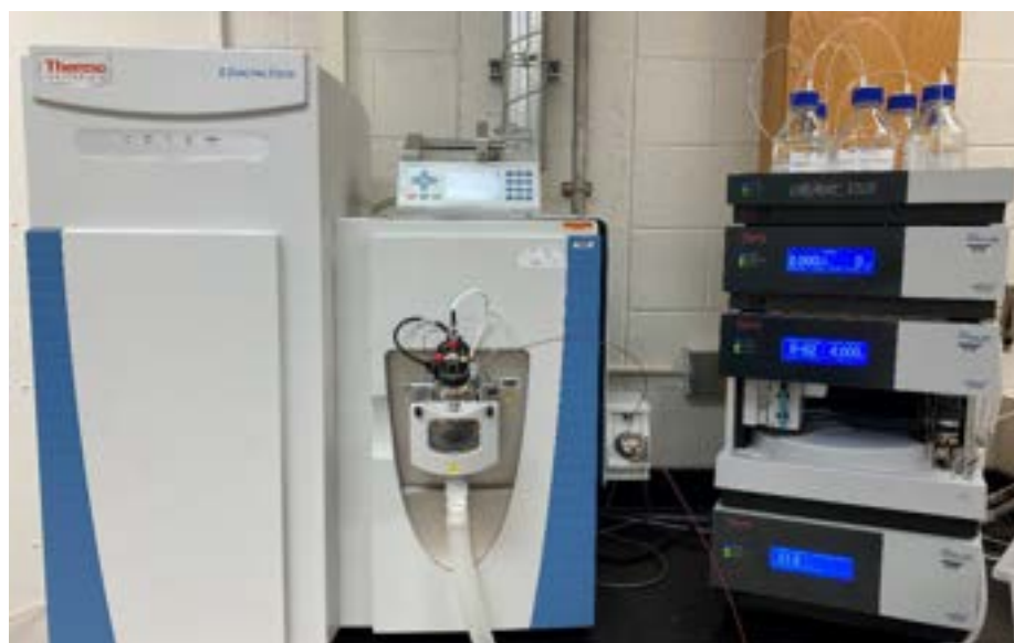
'QE Focus 1' = Thermo Fisher Scientific Q Exactive Focus Mass Spectrometer with UltiMate 3000 UHPLC System
